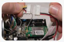
**Step 2:** Unplug the 7-pin power cable connector from the mainboard. Now connect this cable with the corresponding connector from the heating element.
