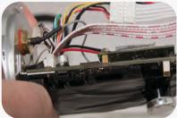
**Step 3:** Connect the other end of the cable from the heating element with the now vacant plug on the mainboard. Now carefully place the element in the lower part of the camera housing. The thermostat of the heating element has to point away from the mainboard.
